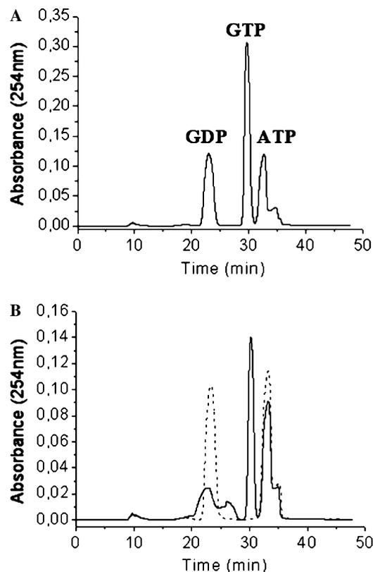
Fig. 5. HPLC-based phosphoryl transferase activity assay for recombinant NDKb. (A) Chromatogram of a 1 mM standard nucleotide mixture containing GDP, GTP, and ATP. (B) Chromatogram of a reaction mixture containing 1 mM ATP and GDP in the absence of enzyme (dashed line) and in the presence of purified recombinant NDKb (solid line). The reactant donor (ATP) and acceptor (GDP) peaks decrease, with the concomitant appearance of the reaction product (GTP).
